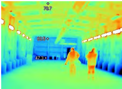
LOW INTENSITY RADIANT HEAT NO SYSTEM-ALL HEATERS ON OUTSIDE 28 °F FLOOR 42°F-- CEILING 90 +°F ALL HEATERS ON
